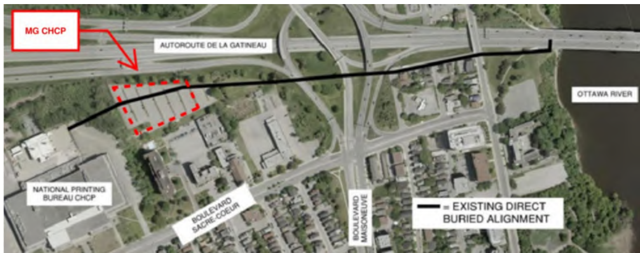
Figure 6.1-1: National Printing Bureau Existing Steam and Condensate Network
