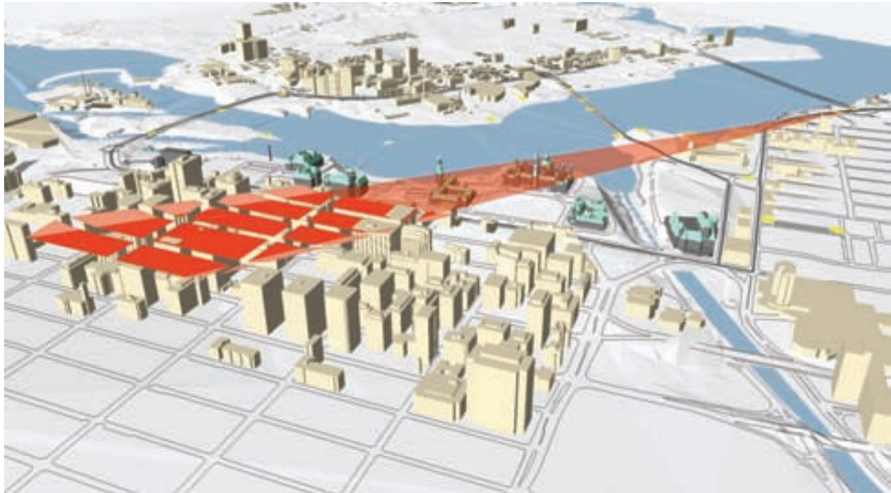
Figure 97: Computer generated image of transition planes
