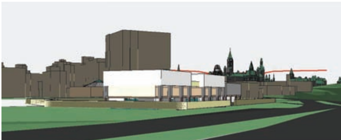
Figure 129: Computer generated view from Viewpoint 1, showing the relationship between the embassy building and the profile of the height planes (red line)
