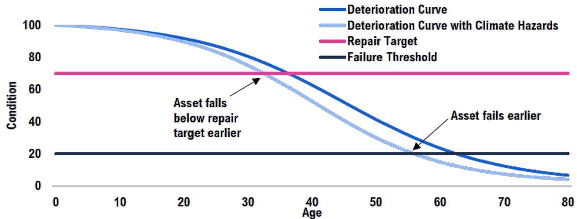
Figure 3. Typical Asset Deterioration Curve with Climate Hazards<sup>13</sup>
