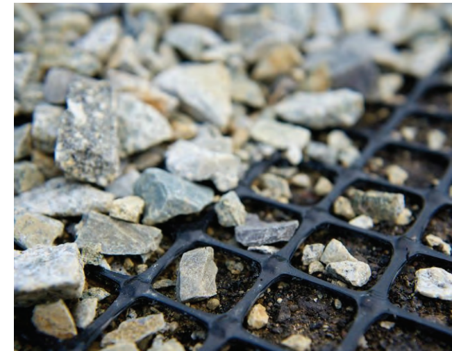
Example of a geogrid-reinforced pathway foundation (see image credits, p.173).
