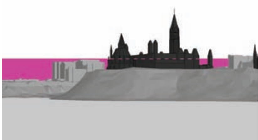
Figure 101: Diagram of control height plane defined by the eavesline of the Centre Block
