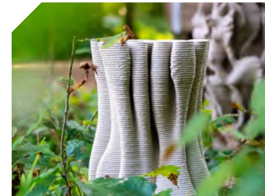
FIGURE 109. 3D PRINTED URBAN MICELIUM REEF FOR BIODIVERSITY Source : Pierre Oskam and Max Latour
