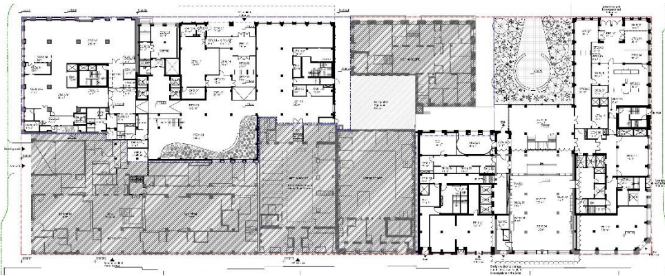
Proposed Ground Floor Plan of Block 2, with out-of-scope portions hatched in diagonally
